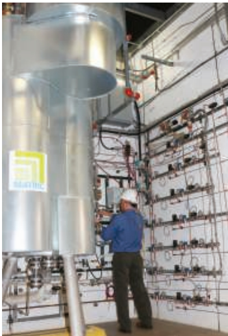
FIGURE 3. Reactor size, as well as instrumentation and analysis requirements, must be taken into account for obtaining accurate cost estimates in pilot plants
