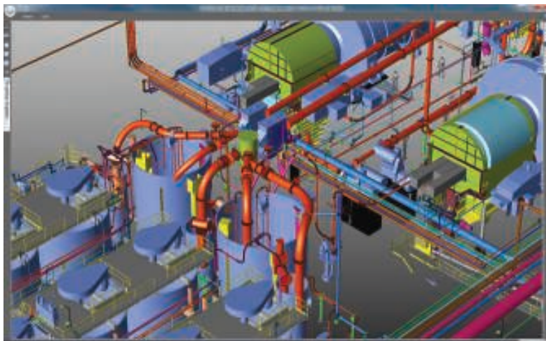
FIGURE 3. The output of a typical 3-D plant layout model is shown here. This model of a solids-handling facility was produced using CADWorx from Intergraph
