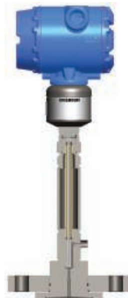
FIGURE 6. In some hot applications, it is required to add additional separation from the process heat to the transmitter. This shows an example cut-away view where the oil fill lines extend to the sensor and protect the temperature of the transmitter
