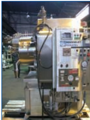
500mm X 250mm Rouselet Robatel Peeler Centrifuge, Hastelloy C22
